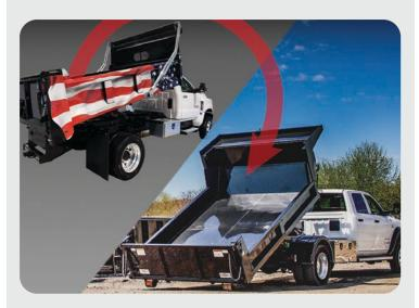
Converting a permanent mount truck to the Switch-N-Go<sup>®</sup> system gives you the ability to use 30+ different interchangeable truck bodies.
