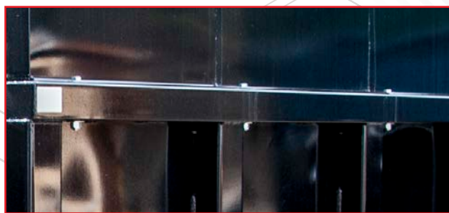
One Piece Roof bolted onto Arbor Body
